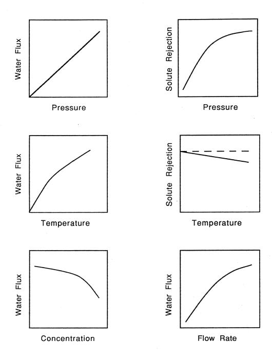
Figure 4. Effects of Variables on RO Separations (Adapted from Riley, 1990).
