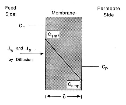
Figure 1. Schematic of a Solution-Diffusion Type Membrane.
