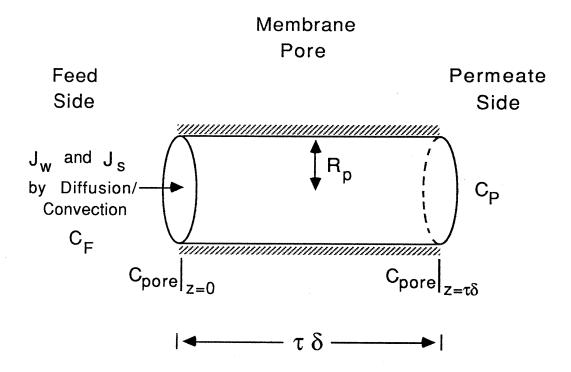
Figure 2. Schematic of a Membrane Pore.
